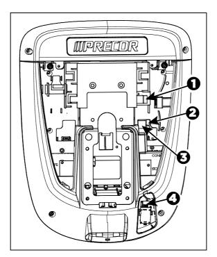
Figure 17: Cable connections, P30 console
